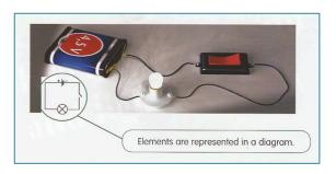
An **electric circuit** is a closed path through which electricity flows. The circuit need to form a complete circle in order to work. We use circuit diagrams to illustrate circuits.
